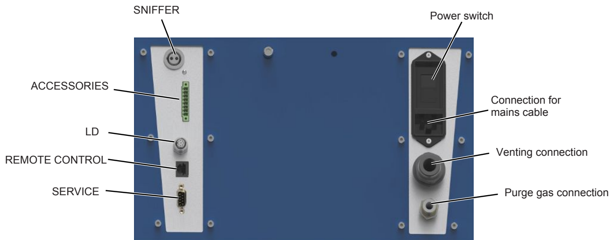
Fig. 6: Connections for accessories and control signals
