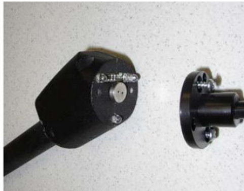
Fig. 18: Sinter filter in the sniffer handle
