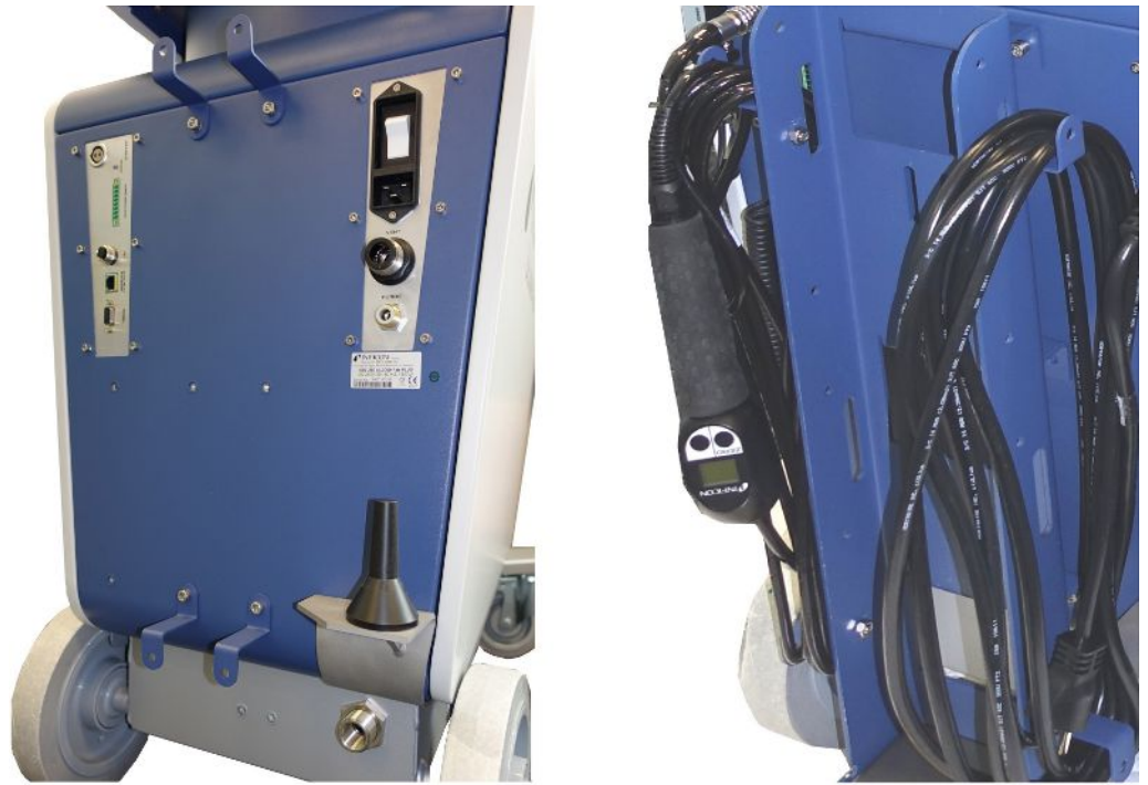
Fig. 7: Hook at the instrument or at the optional bottle holder.
