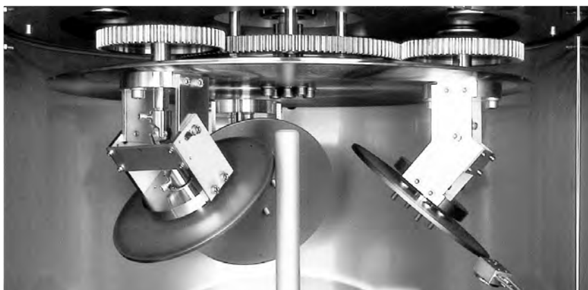
Planetary drive with gear drive and three planets, firmly installed, but where the angle is adjustable
