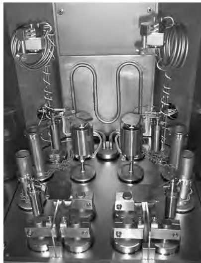
At the foreground: two double thermal evaporators with source shutters In the background: two organics evaporators with source shutters and two film thickness gauge heads
