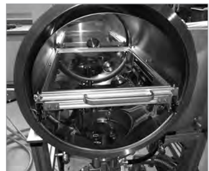
View into the chamber with thermal evaporator and positioned substrate receiver
