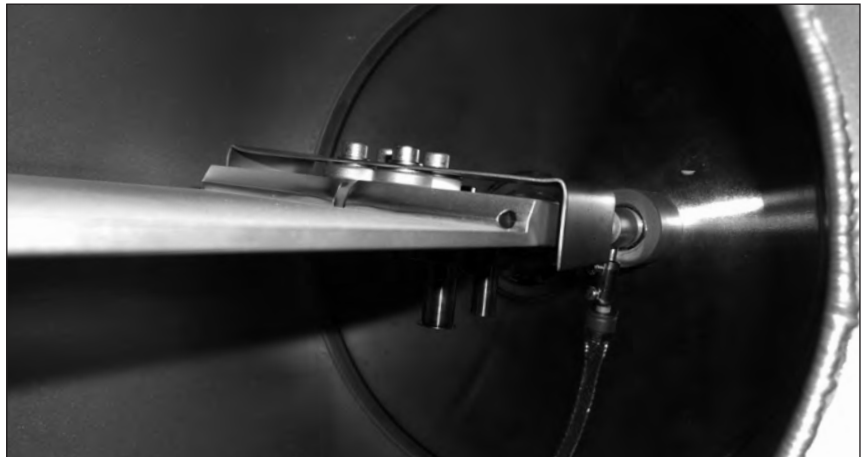
Insulated substrate fork with RF bias connection
