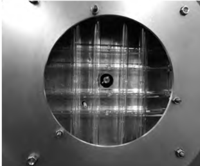
Rotatable thermal radiation heater with quartz lamps
