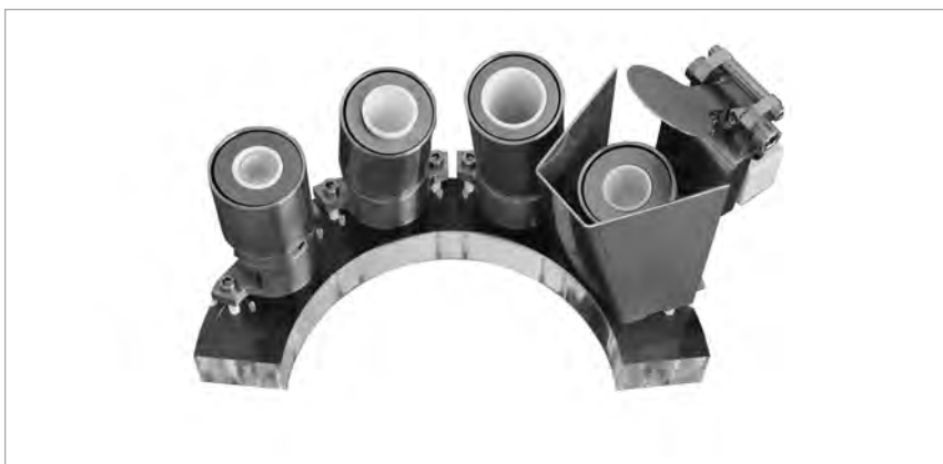
Four organic material evaporators, arranged in a semicircle
