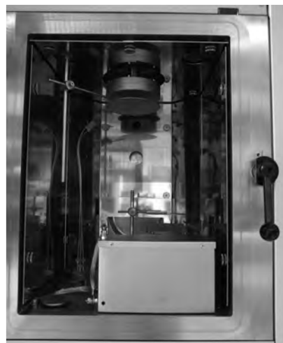
Rotating and water-cooled substrate table
