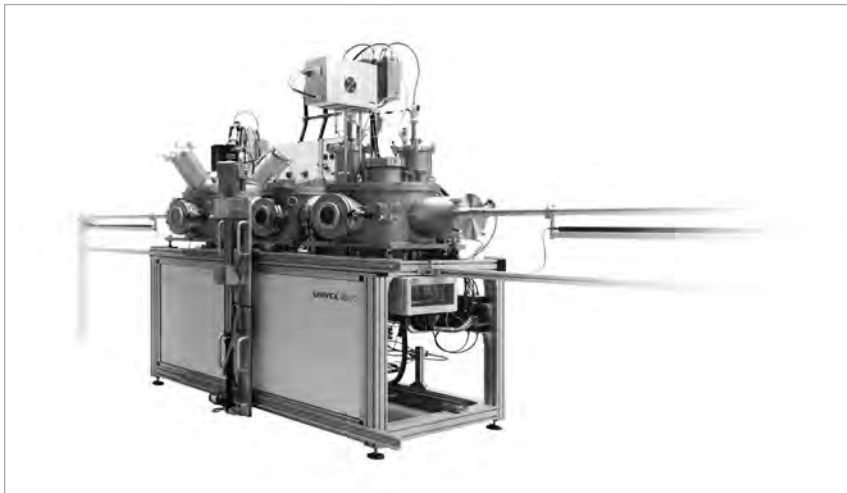
Design example: UNIVEX 450 C with two process chambers as well as load lock chamber arranged at the centre. The substrates are moved using linear transfer rods (left and right)
