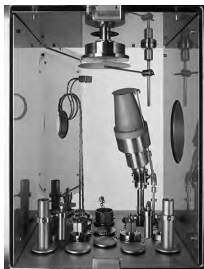
View through the vacuum chamber: front sliding door and rear swivelling door open Design example with sputter source (right) and heated substrate table (top)
